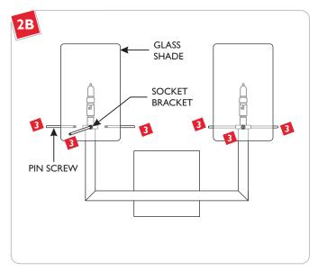
3 Align the glass shade holes with the socket bracket holes and tighten the four pin screws to secure the glass shade in place.
