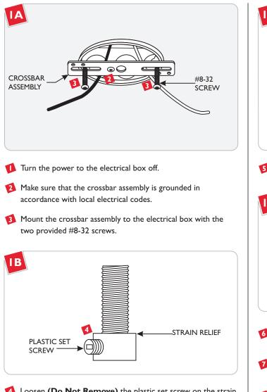
Loosen (**Do Not Remove**) the plastic set screw on the strain relief.
