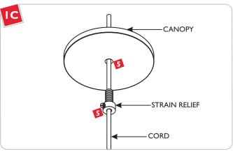
5 Feed the cord through the strain relief and the canopy.
