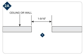
• Use a 1-9/16" hole saw to cut out the ceiling or wall where the ports are going to be installed.
