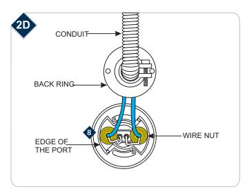
Place the wire nut connections and the port wires properly inside the port. Make sure that the port and low voltage wires are cleared from the edge of the port.
