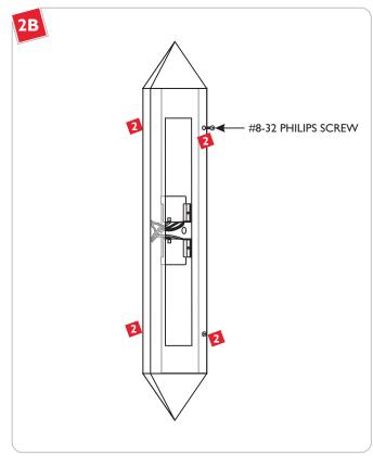
Align the metal shade holes to the mounting plate side holes. Replace and tighten the four #8-32 Philip screws to secure the metal shade in place.
