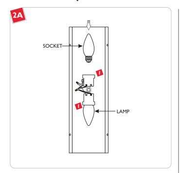
Use **MAX 40** Watt Type B13 Medium Base Torpedo Lamp With Each Socket.
