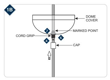
**NOTE:** Refer to the instructions provided with the pendant fixture to install the fixture shade (if needed) before proceeding with these steps.
