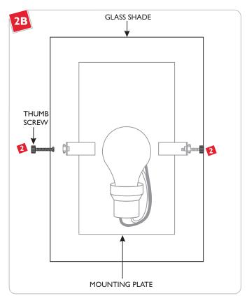
2 Place the glass shade onto the mounting plate. Align the glass shade holes with the mounting plate holes. Tighten the thumb screws to secure the glass shade in place.
