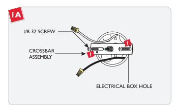
Mount the crossbar assembly to the electrical box holes with the two #8-32 screws provided.
