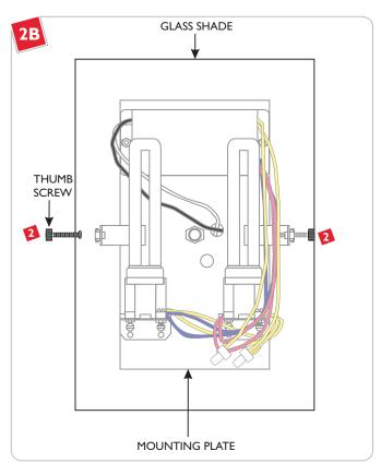
Place the glass shade onto the mounting plate. Align the glass shade holes with the mounting plate holes. Tighten the thumb screws to secure the glass shade in place.
