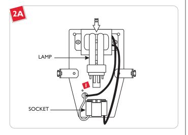
Use **MAX 13** Watt Type Quad Tube GX23-2 Base Compact Fluorescent Lamp.
