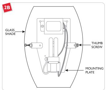
2 Place the glass shade onto the mounting plate. Align the glass shade holes with the mounting plate holes. Tighten the thumb screws to secure the glass shade in place.
