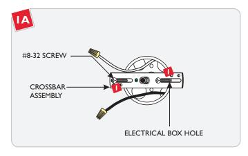
Mount the crossbar assembly to the electrical box holes with the two #8-32 screws provided.
