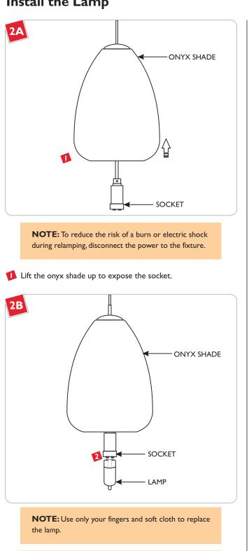
Use MAX 50 Watt, Type Xelogen (Xenon) Bi-Pin Lamp.
