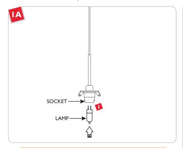
NOTE: To reduce the risk of a burn or electric shock during relamping, disconnect the power to the fixture.
