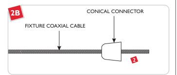
2 Insert the fixture coaxial cable through the conical connector.
