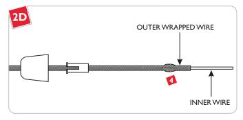
**1** Slide the outer wrapped wire back to expose the inner wire.
