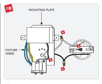
Feed the fixture wires through the mounting plate side hole.
