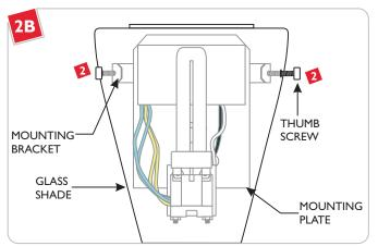
2 Place the glass shade onto the mounting plate. Align the glass shade holes with the mounting plate holes. Tighten the thumb screws to secure the glass shade in place.
