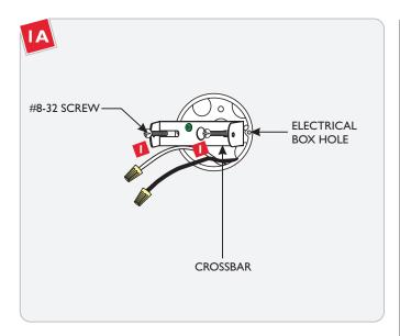
Mount the crossbar to the electrical box holes with the two #8-32 screws provided.
