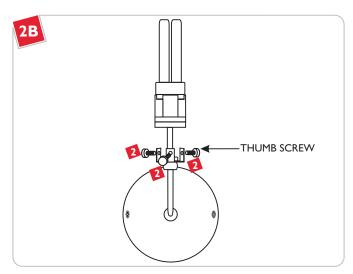
Remove the three thumb screw.
