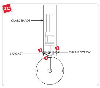
Align the glass holes with the bracket holes. Replace and tighten the three thumb screws to secure the glass shade in place.
