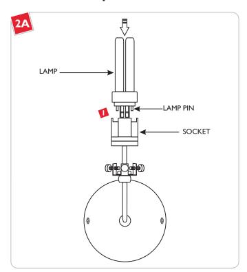
Use MAX 13 Watt Type Quad Tube GX23-2 Base Compact Fluorescent Lamp.
