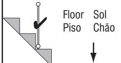
If the gate is used at the bottom of the stairs to prevent the child from climbing up the stairs, it must be placed on the lowest stair.
