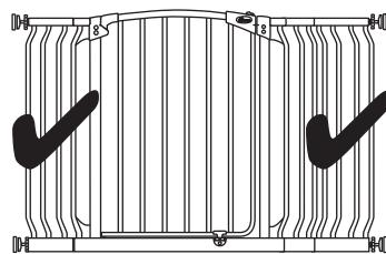
**WARNING:** A maximum of 4 Gate Extensions can be used, 2 on either side of gate. Do NOT install 3 Gate Extensions on the same side of gate.
