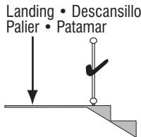
**WARNING!** Hardware mount the mounting cups when using gate at the top of the stairs.
