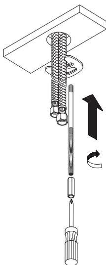
3. Attach rubber washer and metal washer onto copper tubes. Screw metal threaded rods onto faucet body.
