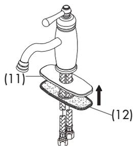
1. Attach cover plate to bottom of faucet with plastic gasket.
