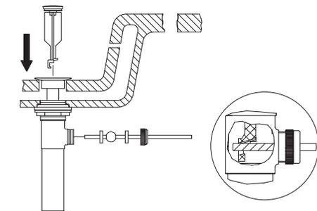
5. Insert stopper assembly (8) into drain. Insert ball rod (5) into rod port and into hole at bottom of main plunger.
