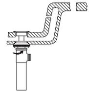
2. Place a ring of silicone sealant around drain opening of sink.
