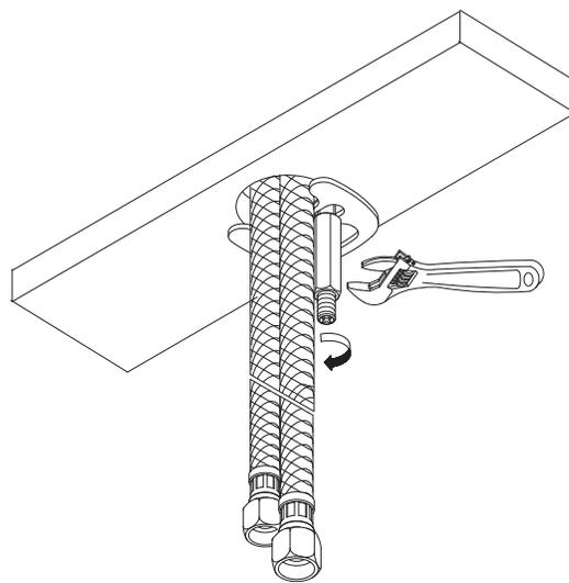
4. Tighten the nut on metal threaded rods.
