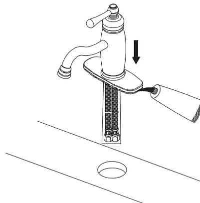
2. Place silicone sealant beneath the plastic gasket and install faucet through center hole.
