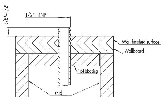
**NOTE:** INSTALL 1" x 4" WOOD BLOCKING BOARD FLUSH TO FRONT OF STUD FACE CENTERED AT FAUCET MOUNTING POINT.
