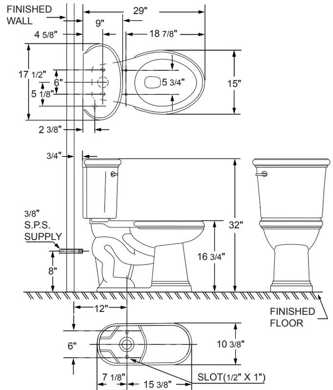
IMPORTANT: Dimensions of fixtures are nominal and may vary within the range of tolerance established by ASME Standard A112.19.2. These measurements are subject to change or cancellation. No responsibility is assumed for use of superseded or voided pages.
