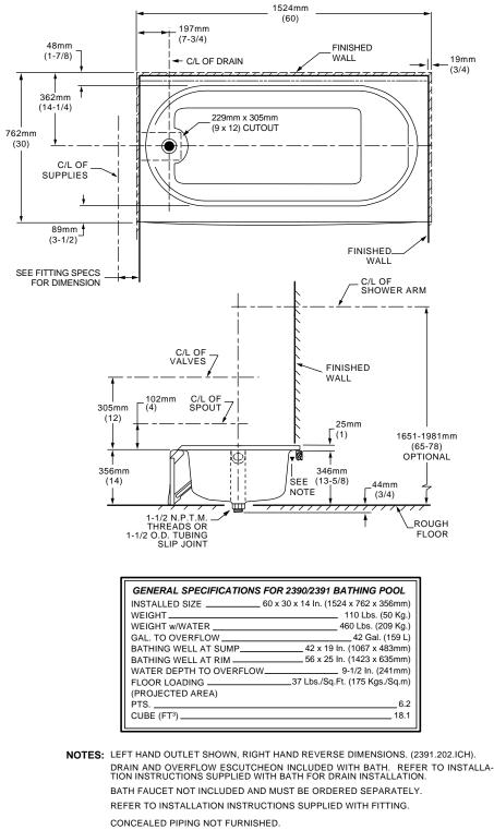
PROVIDE SUITABLE REINFORCEMENT FOR ALL WALL SUPPORTS. ▼ REFER TO INSTALLATION INSTRUCTIONS SUPPLIED WITH BATH.
