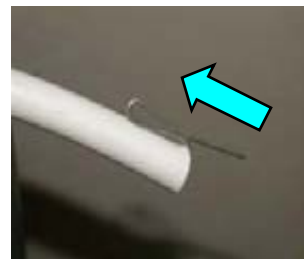
Re-insert the "S" clip into the end of the refill tube.
