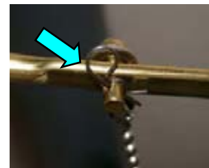
Re-insert the hair pin cotter through the clevis pin hole.
