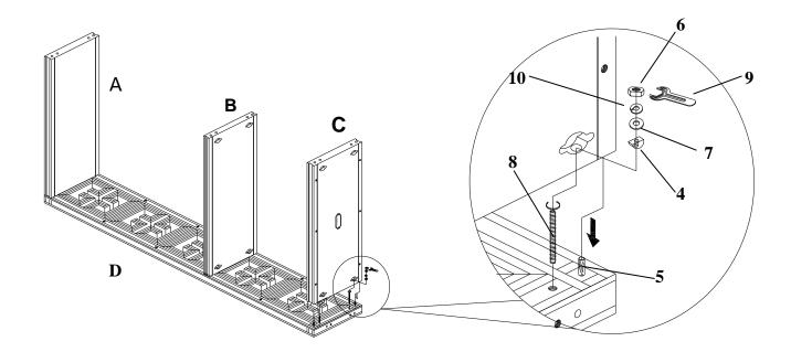
Caution: The side with holes for the Top panel (A) must face upward. The side with holes for the Fixed panel (B) and Bottom panel (C) must face downward.
