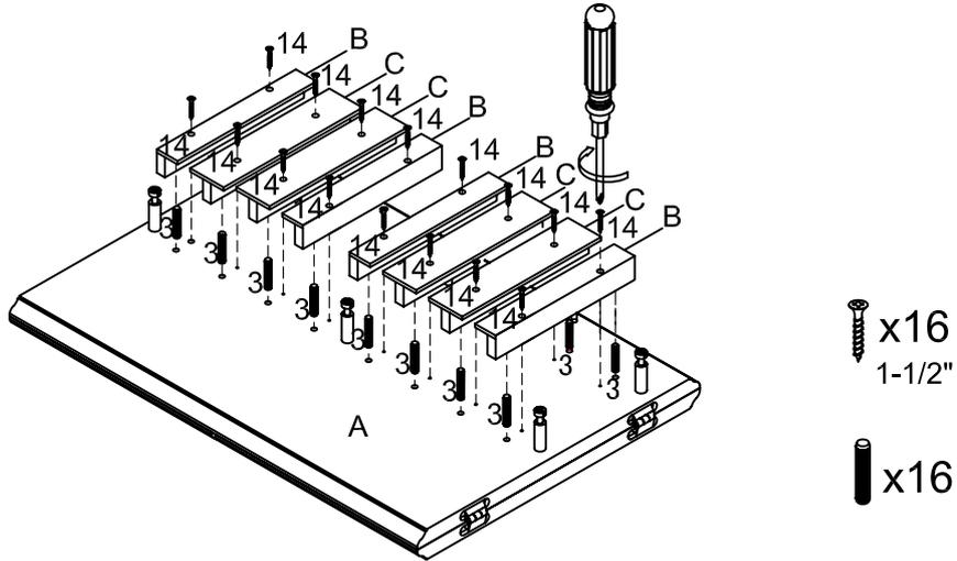
Step 7. Attach Expandable Top A to Parts D, E, F, & I with Wood Dowels & Cam Locks as shown. Secure Rail X to Expandable Top A with Screw (Part #4) using Phillips Head screwdriver as shown.
