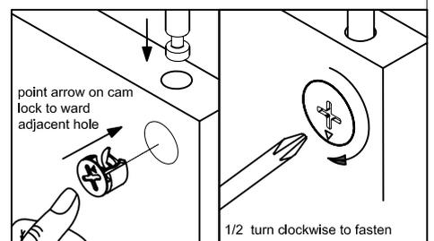
Step 4. Attach Front Panel I to Parts D & F using Cam Locks as shown.
