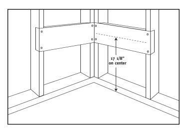
1. The shower seat must be installed using sufficient inwall backing materials. A 2 x 6 wall support must be installed 17-1/8" on center. This will provide a shower seat height of approximately 19".
