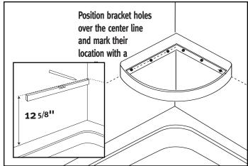
2. A common shower seat height is 19". To accommodate this suggested height, mount the wall bracket 12-5/8" off of the shoulder of the Swanstone Shower Floor. If mounting over a Swanstone Retrofit Shower Floor, the 12-5/8" measurement must be changed to 13-5/8" or 17-1/8" off of the subfloor.
