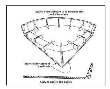
5. Apply silicone adhesive (supplied) to the mounting tabs on the underside of the seat as illustrated.
