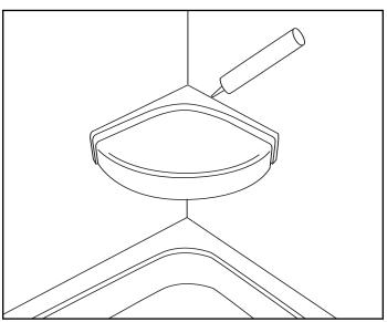
6. Set the shower seat into place and clean any excess silicone from the wall or seat surface. It may be necessary to re-caulk around the outer perimeter of the shower seat. Following installation, silicone adhesive residue can be cleaned with mineral spirits.
