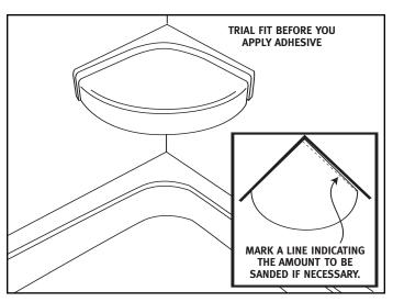
4. Trial Fit — Prior to applying adhesive, set the shower seat into position. This will insure that it will fit tightly against the wall. If the wall is not exactly 90 degrees square, it will be necessary to sand one side in order to achieve proper fit. Use a coarse grit (60 grit) sandpaper.
