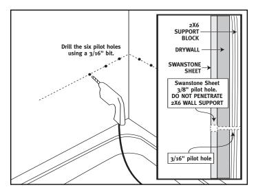
3. Drill six pilot holes using a 3/16" drill bit.
