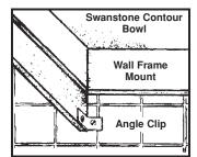
Drill a 1/32" pilot hole (3/8" deep) into the Swanstone apron panel and mount angle clip to the apron panel with
