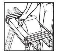
pilot hole from the underside. Drill fixture holes from the top side with a 1-1/4" router, spade bit, twist drill or hole saw. Do not use an auger bit. Faucets may be installed at this time.
