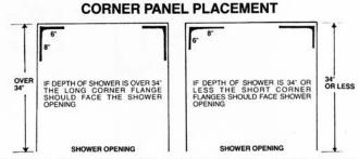
DO NOT NAIL PANELS TO SUBWALLS. THE HOLES IN THE CORNER PANELS ARE FOR MANUFACTURING PURPOSES ONLY!
