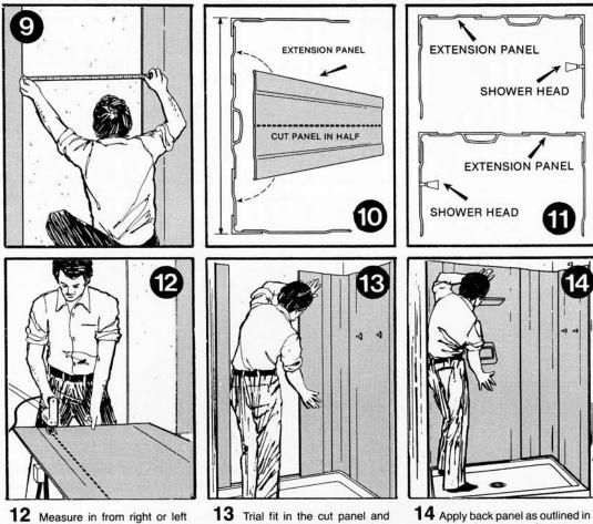
**12** Measure in from right or left hand edge depending on location of outlets and mark. Cut with saber saw.
