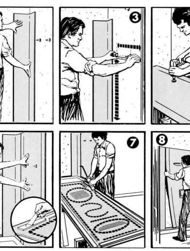
**6** Remove backing from factory applied pressure sensitive tape. Grasp side panels by the edges, carefully position by **overlapping** the corner panel. Press firmly from top to bottom, then press the entire surface the same way to insure solid wall contact.
