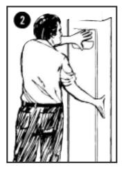
2. Carefully position corner panel and press it firmly to the wall. Move hand pressure up and down and side-to-side making sure all areas are in firm contact with the wall. Repeat steps 1 and 2 for the other corner panel.
