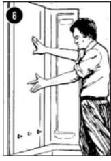
Use even pressure from top to bottom and side-to-side to insure solid wall contact. Install other side panel and back panel in like manner.
