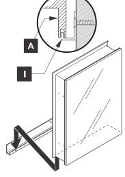
With assistance, rest the cabinet on the mounting bar and hold in place.
