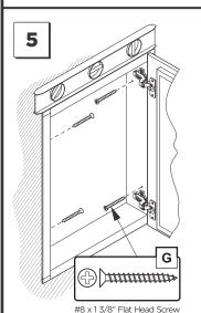
Level, then secure the cabinet with screws (G) through the mounting holes into the framing studs.
