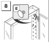
Fill remaining holes with the plugs (**E**).
