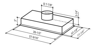
Mount power pack so bottom of unit is 24" to 30" above cooking surface.
