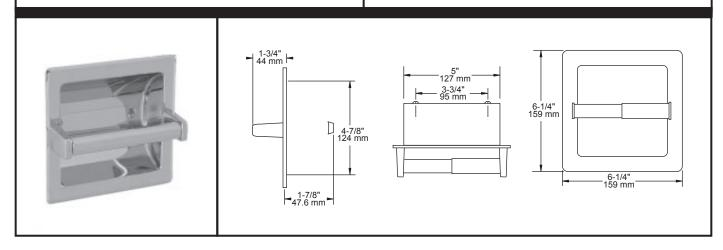
MATERIALS: Chrome plated recessed shells are stamped from 21 gauge special alloy brass strip, highly polished and chrome plated. Stainless steel
