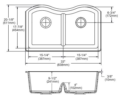
(NOT FURNISHED) COUNTERTOP REVEAL APPROX. 1/8" MOUNTING CLIP SINK **FASTENER** (NOT FURNISHED) Cross Profile of Installation For Sinks Purchased Prior To Apr. 1, 2013 Template 74180592 (available by contacting customer service) SILICONE CAULK (NOT FURNISHED) COUNTERTOP
