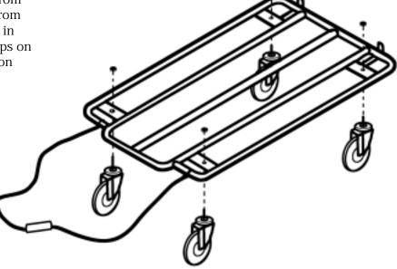
**2.** Check to make sure all four wheels are level. Thread a large washer, smaller lockwasher and nut onto each wheel bolt. Tighten nuts securely.
