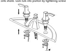
Remove flange (1) and rubber washer (2) from POP-UP drain assembly.
