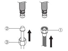
Slide Hot and Cold end valves thru sink mounting holes. NOTE:Hot side end valve is labeled. Secure end valves with washers and nuts. Hand tighten nuts onto shank. Lock nuts into pisition by tightening screws.
