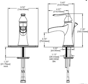
NOTE: 1. All dimensions are in inches (millimeters) unless otherwise specified and are subject to change without notice. 2. Flex hoses have 3/8 compression female threaded connections.
